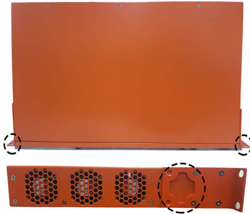
Figure 15 Rack Bracket Installed for Extra Space
